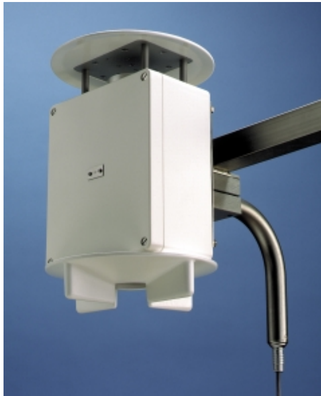
Thermohygrometer VTP 6 mounted electrically insulated on a meteorological mast outrigger. The air intake is visible at the bottom. The air leaves the housing through a duct below the lid.
