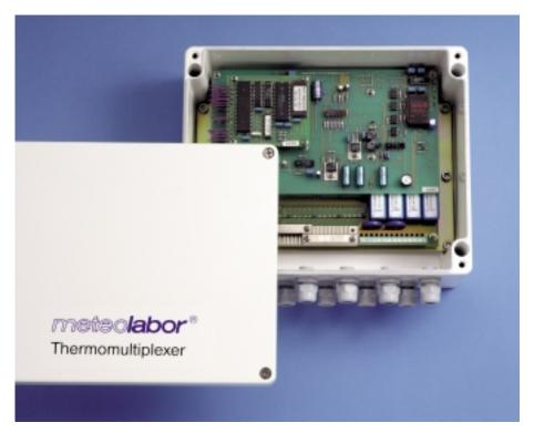
The thermomultiplexer TMUX is a universal thermometer with an RS232 / RS485 interface. It has 30 channels for temperature measurement using thermoelements as temperature sensors. The thermoelement technique allows not only temperature measurement at a given point, but also enables determination of the temperature difference between any two points.
