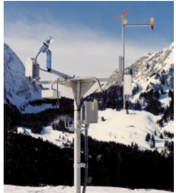
Meteorological sensors for wind speed and wind direction, illuminance, radiation, and temperature near Einsiedeln
