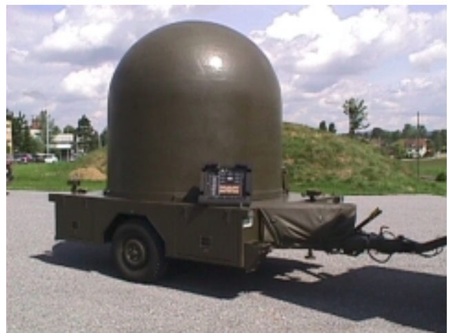
TE: Telemetry unit, containing tracking antenna and the electronic circuits for telemetry
